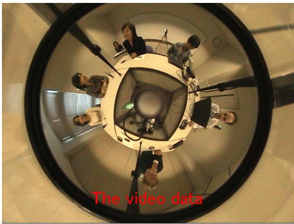
Figure 1: A 360-degree camera provides a view of all participants at the meeting, and although the resolution is low, their body movements can be tracked using skin-tone-sensitive image processing algorithms (see fig 3)
